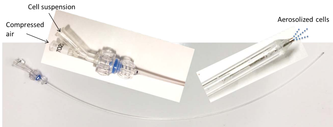
Figure 1: Microjet™ Sprayer optimized for high cell viability and access in decellularized lungs
